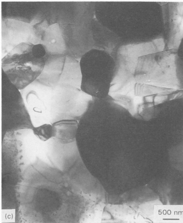
Figure 10 Transmission electron micrographs of 30 vol % \text{Cr}_3\text{C}_2/\text{Al}_2\text{O}_3 composites after oxidation at 1200 °C; (a) the oxidized layer, \text{Cr}_3\text{C}_2 completely oxidized to form micropores; (b) next to the oxidized layer, \text{Cr}_3\text{C}_2 partially oxidized; (c) the unoxidized region, \text{Cr}_3\text{C}_2 are black particles, \text{Al}_2\text{O}_3 matrix is grey. Microvoids and micropores are white.
