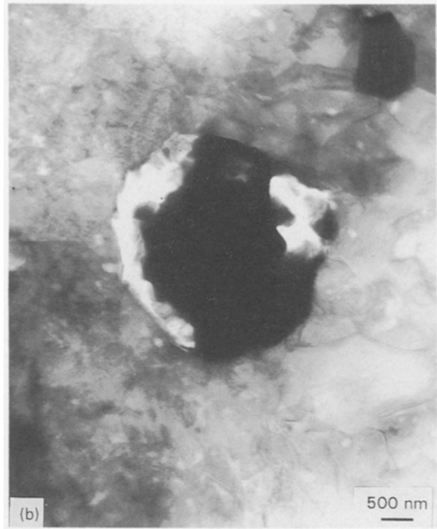
Figure 10 Transmission electron micrographs of 30 vol % \text{Cr}_3\text{C}_2/\text{Al}_2\text{O}_3 composites after oxidation at 1200 °C; (a) the oxidized layer, \text{Cr}_3\text{C}_2 completely oxidized to form micropores; (b) next to the oxidized layer, \text{Cr}_3\text{C}_2 partially oxidized; (c) the unoxidized region, \text{Cr}_3\text{C}_2 are black particles, \text{Al}_2\text{O}_3 matrix is grey. Microvoids and micropores are white.
